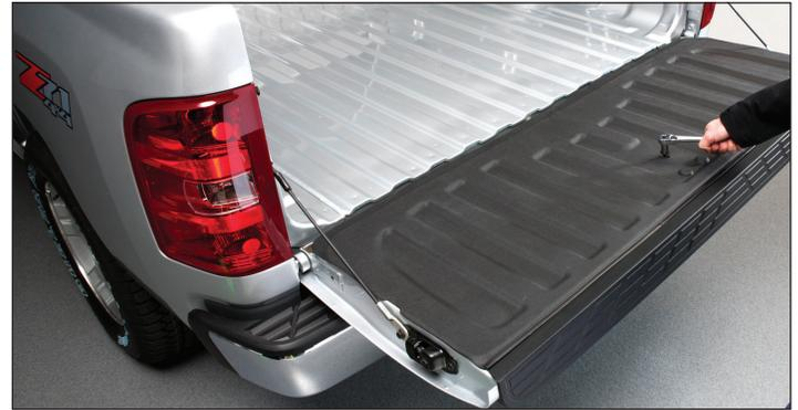
**6** Once the Tailgate Techliner™ is in place, take the bolt and washer that you previously removed and re-install them over the Tailgate Techliner™. DO NOT OVER TIGHTEN.
