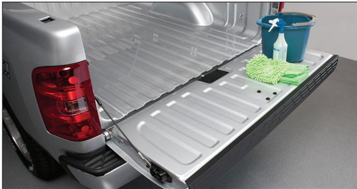
**1** Lower the tailgate and remove all tailgate accessories prior to installation. Clean your truck bed and tailgate with soap and water or TechCare™ Gentle Car™ Shampoo and dry thoroughly before installing the Tailgate TechLiner™.
