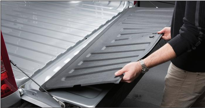
**5** Lay the Tailgate TechLiner™, Velcro® pads facing down, onto the tailgate making certain the features align.
