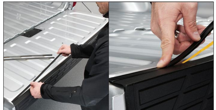
**4** Remove the three plastic extrusions from the parts bag. Place the first extrusion against the edge with the opening facing the front of the vehicle. Slowly remove the adhesive backing, pressing firmly as you go.
