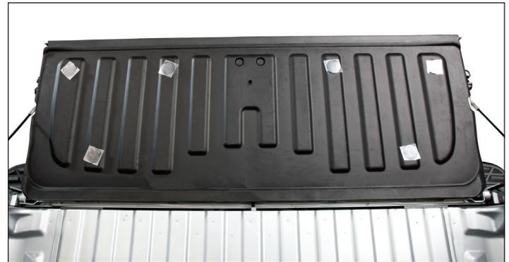
**2** Place Tailgate TechLiner™ on a dry, flat surface\*. Unfold and lay out to allow liner to flatten. (For faster results, lay liner in the sun and put a small weight on each of the corners.)
