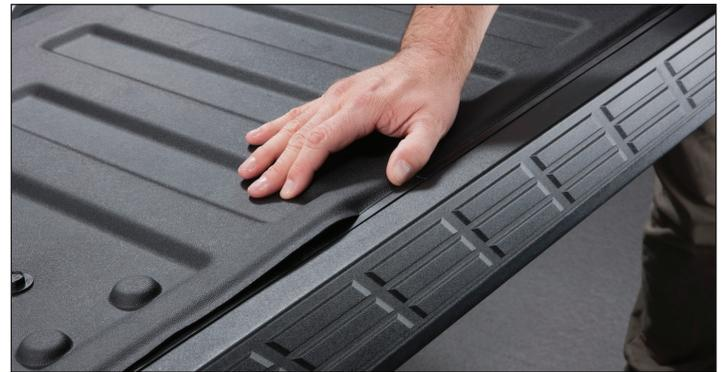
**8** Starting at one end, begin tucking the edge of the Tailgate Techliner™ into the plastic extrusion that you previously installed. Work your way down the entire length of the tailgate.
