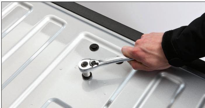
**3** Use a socket or wrench to remove the center bolt and washer from the tailgate as shown. Retain this because you will use it again in a later step.
