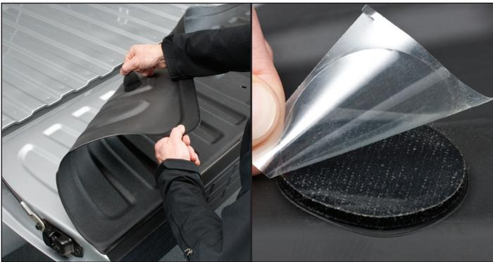
**7** Bend the Tailgate TechLiner™ backward to locate the first Velcro® disc without shifting the position of the Tailgate TechLiner™. Remove the backing from the Velcro® disc and fold the tailgate TechLiner™ back into place. Press down firmly on the location of the Velcro® disc. Continue the process in a clockwise direction.
