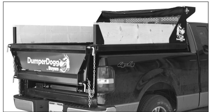
1. Use existing hole and (1) hex head cap screw to position rear bracket assemblies (Fig. 1).
