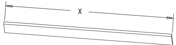
Measure Between Inside Of Front And Rear Brackets To Obtain Length "X" For The Necessary Length Of Board
