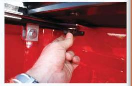
STEP 5: fold cover shut to ensure a propper fit. Adjust if necessary.
