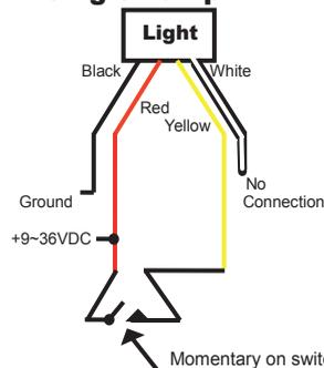
Make connections as in Step 1 & 2. The white wire is not used for a single lamp installation.
