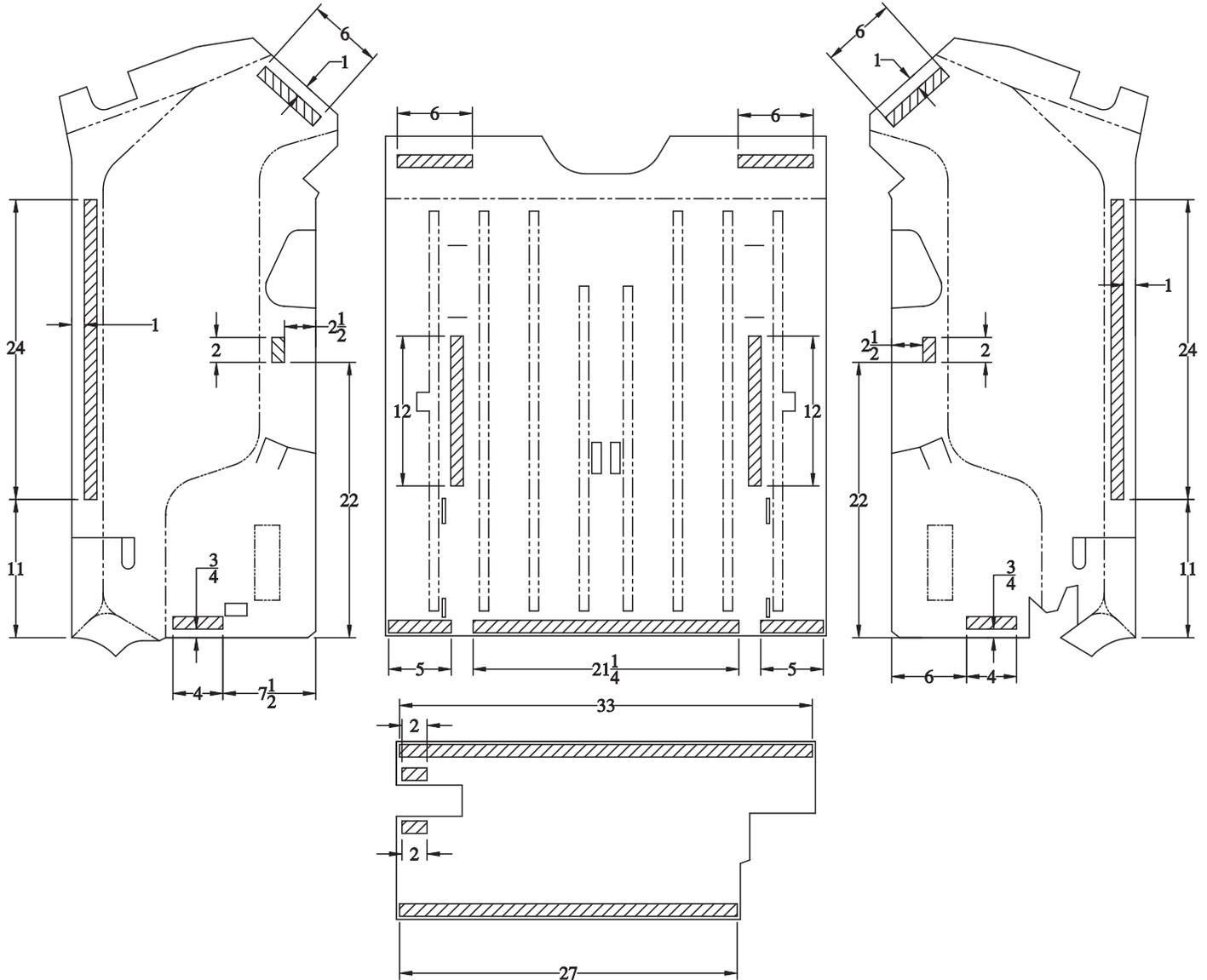
**Note:** Cargo floor has high cycle loop fasteners pre-installed at the factory in locations noted on the drawing. Apply hook fasteners to these pre-installed loop fasteners.
