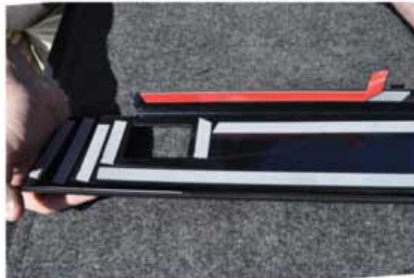
5. On the sides, partially peel (dog ear) tape so it can be easily accessed from the bottom of the rail
