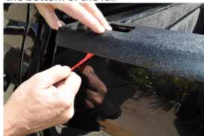
8. Do the same along the outer rail and make sure to apply pressure for the tape to take hold
