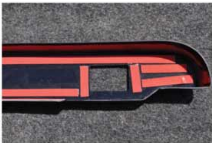
4. Remove the red protector from the 3m tape on the TOP surface ONLY
