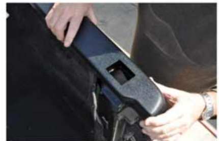
6. Set the ProCap straight down on the truck bed rail. Set alignment before sticking down.
