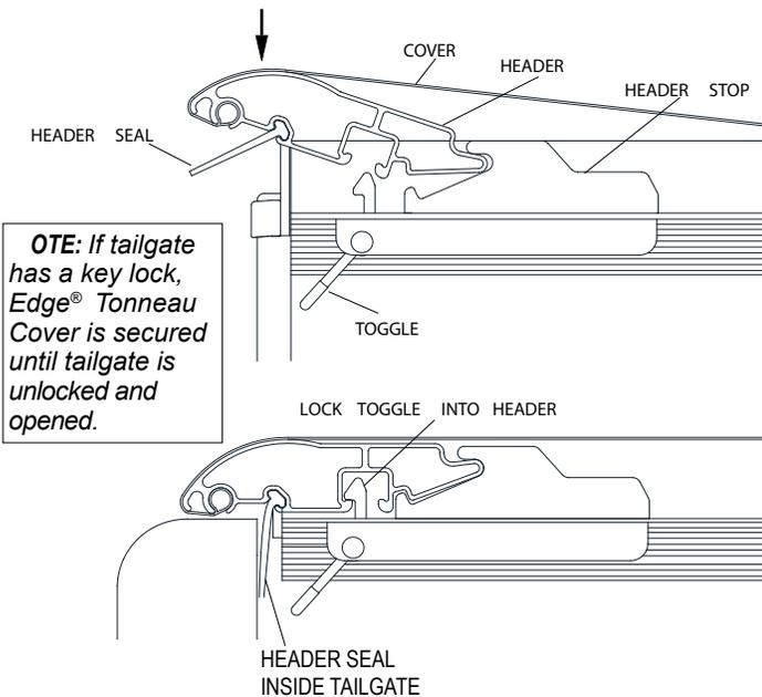
**OTE:** If tailgate has a key lock, Edge® Tonneau Cover is secured until tailgate is unlocked and opened.
