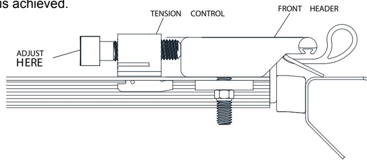
**NOTE:** Adjust tension in small increments. Slight adjustments yield significant results.
