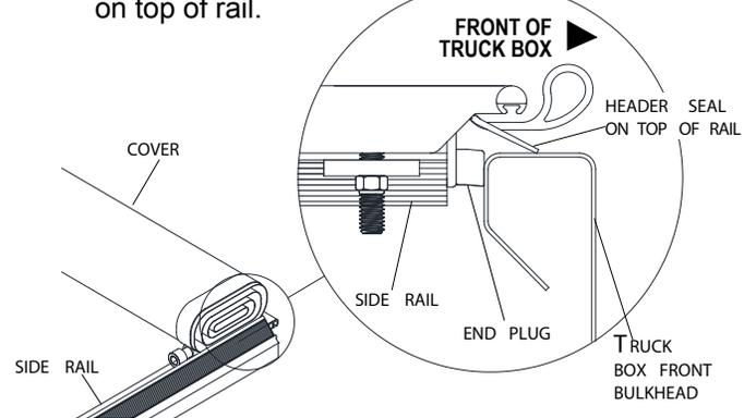
**STEP 5:** Tighten bolts but do not over tighten. Header must be free to slide.
