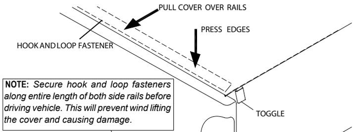
**NOTE:** Secure hook and loop fasteners along entire length of both side rails before driving vehicle. This will prevent wind lifting the cover and causing damage.
