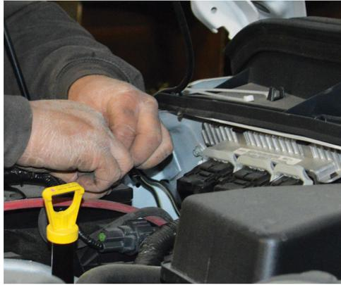
**5a.** Next, connect the power cable from the solenoid to a positive power source. Wire a 4 gauge ground from the winch motor directly to the negative terminal of the truck battery using the PS501R.
