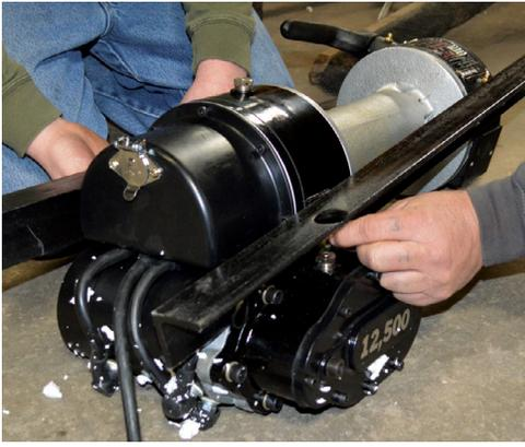
**1.** After removing the winch from the box, install the angle mounts onto the winch frame.
