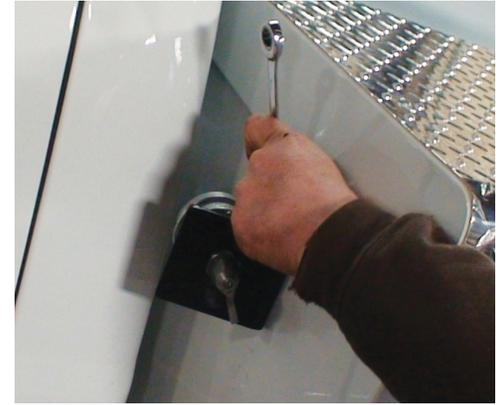
**5b.** Also, install and connect the safety cutoff switch at any easy, reachable distance from the winch. The cable we used was the PS501.
